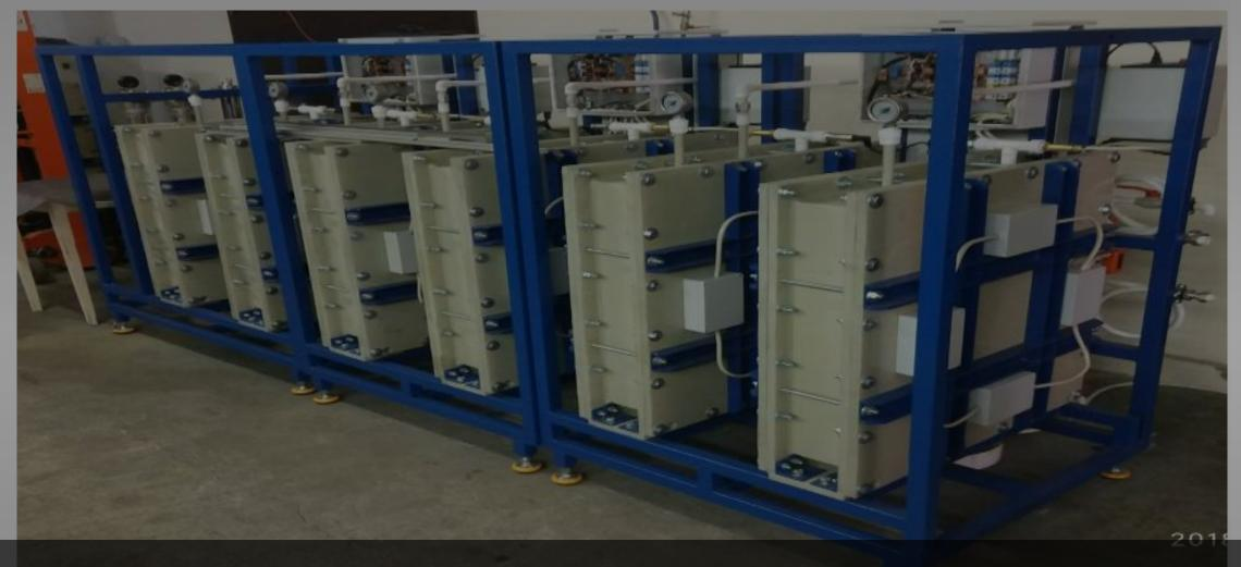
Deionize water by applying an electrical potential difference over two electrodes.
